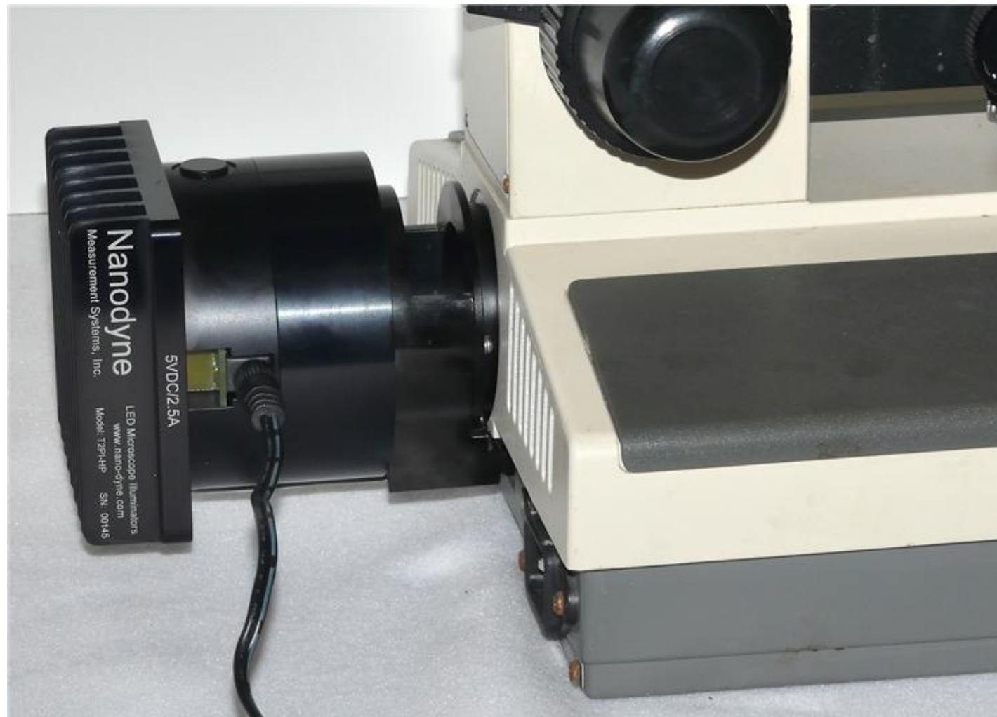
Connect the power cable to the illuminator and power supply. Plug the power supply into an AC outlet and the system is ready to operate. There is no off switch. The LED is completely off when the control is slid back towards the front of the microscope.
