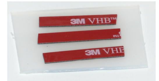
Tape to secure wires.
